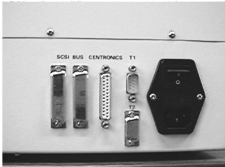
When connecting the cables please pay attention, that all interface- and/or power cables are grounded properly and that they are in accordance with the electronically regulations.
